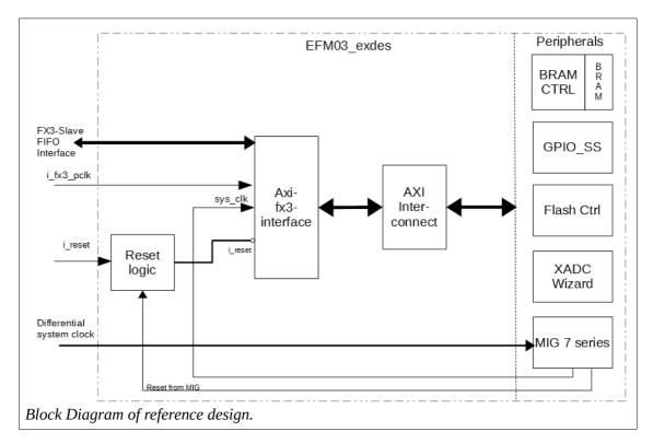
The reference design receives commands from the host, and based on the received command, performs a READ or a WRITE operation on the addressed peripheral. A brief explanation is provided below about the components used.
