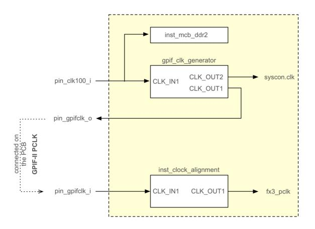
At pin\_gpifclk\_i (LOC = Y12), the efm02\_soc reference design expects the externally reefed clock signal PCLK of the GPIF-II interface. To compensate routing and buffer delays, it is aligned by inst\_clock\_alignment. The aligned clock fx3\_pclk sources the GPIF - Wishbone interface wb\_ma\_fx3.vhd
